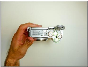
Unlock the battery cover, while swinging the cover outward to open it.
