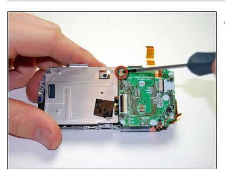
Remove the 2.5 mm silver screw from the upper left corner of the motherboard.
