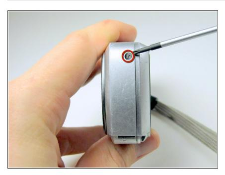
Locate the 5.3mm silver screw on the edge closest to the upper left corner of the LCD screen and remove it.
