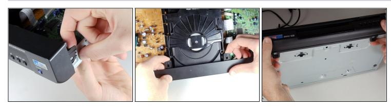
• There are six symmetrically placed tabs holding in the front faceplate. Unhook these six tabs to loosen the faceplate.
