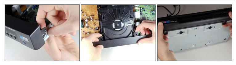
• There are six symmetrically placed tabs holding in the front faceplate. Unhook these six tabs to loosen the faceplate.
