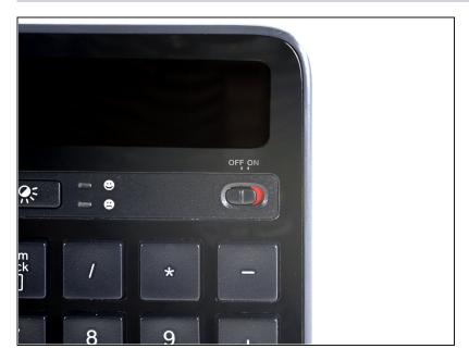
Before you begin, flip the keyboard's power switch into the **OFF** position.
