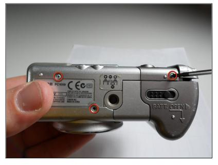
Remove the three Phillips #00 screws from the bottom of the camera.
