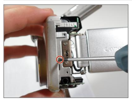
Using the Phillips #00 screwdriver, unscrew the 2.4 mm long screw that holds on the front panel underneath the side panel.
