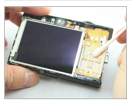
Clean around the function buttons with a cotton swab dipped in isopropyl alcohol.
