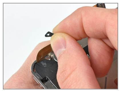
Remove the small black spacer that was under the Phillips screw near the vibrator.
