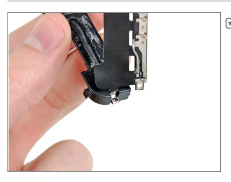
When installing a new cellular antenna, be sure to slide the gold bracket over the ear molded into the speaker enclosure before sticking the antenna down.
