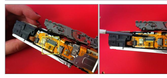
Using the spudger, flip the clip in an upward motion. The clip should remain attached to camera, not removed completely.
