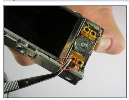
Using tweezers, gently slide the LCD cable, horizontally from its white plug towards the camera screen.
