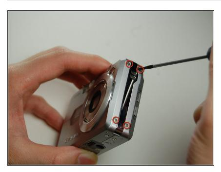
Using the Phillips #00 screwdriver, remove the four screws from the side of the speaker.
