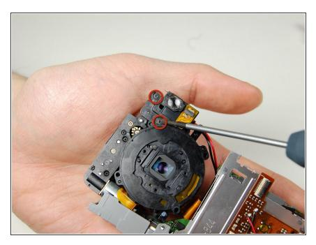
On the backside of the camera where the indicator lamp is located, remove the two screws using the Phillips #00 screwdriver.
