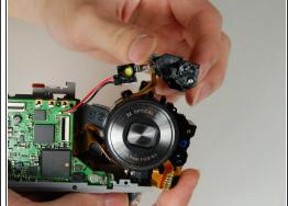
• On the front side of the indicator lamp remove the screw using the Phillips #00 screwdriver.
