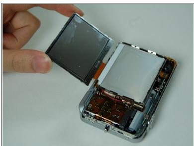
Lift the LCD screen and move it to the other side.
