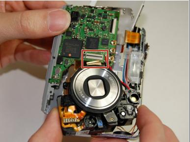
Flip the connector and remove the ribbon cable from the motherboard next to the lens.
