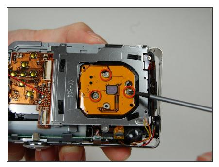
On the back of the camera where the LCD screen was, remove the 3 screws located behind the lens using the Phillips #00 screwdriver.
