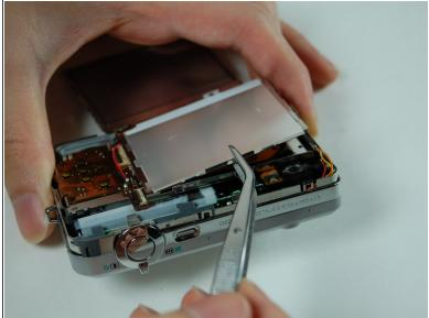
Using a pair of tweezers, pry off the LCD casing.
