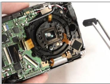
• Using <u>tweezers</u>, remove the cylindrical gear from the camera.
