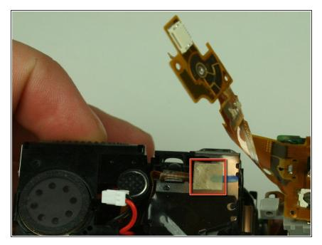
Adhesive tape attaches the flex circuit to the top of the camera.
