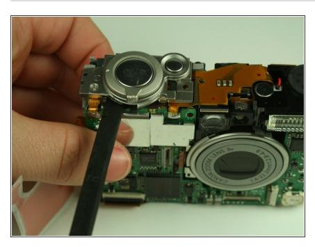
Using a spudger, carefully pry the shutter button assembly from the camera.
