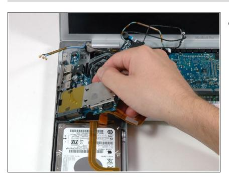
Lift up the right side of the left I/O board and slide it out of the computer.
