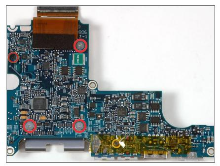
Remove the four Phillips screws securing the ExpressCard cage to the left I/O board.
