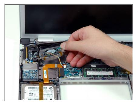
Lift the left fan up and carefully peel up the tape securing the fan to the heat sink as you go.
