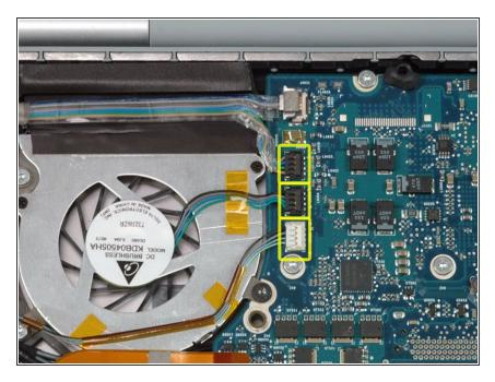
Disconnect the inverter, left fan, and left ambient light sensor cables by placing a spudger beneath each cable and lifting up.
