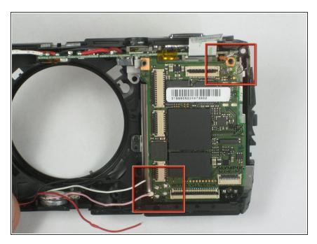
Desolder the upper right and lower left wires to remove the motherboard.
