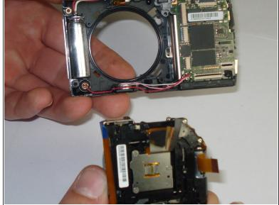
• Using your thumb and forefinger, pull the lens piece straight out from the body of the camera.
