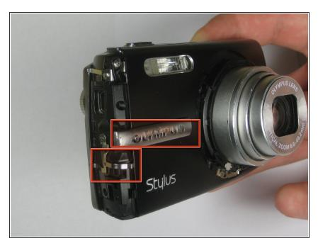
Using your thumb and forefinger, pull off the silver name plate and silver "T-shape" piece.
