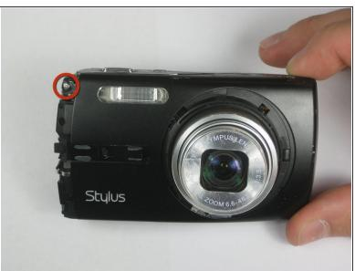
Remove the remaining three Phillips #00 side and front panel screws.
