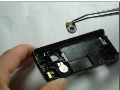
Remove the speaker by pulling it up and out of place with the tweezers.
