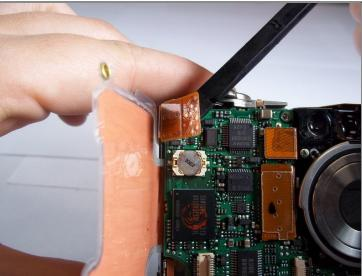
• Remove the ribbon cable on the top left corner of the motherboard by using the flat end of the spudger to pry the cable from the board.
