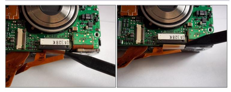
• Insert the pointed end of the spudger under the ribbon cable and gently pull the cable out of its port.
