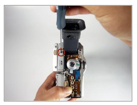
Remove the 4mm #00 Phillips screw located to the right of the LCD release switch.
