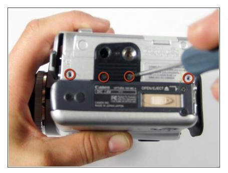
Remove the 4 Philips #00 4mm screws shown.
