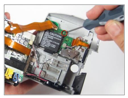
• Remove the screw above the speaker's housing.
