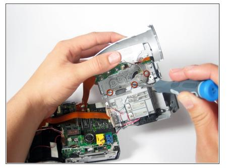
• Remove the 3 screws holding the metal piece over the speaker.
