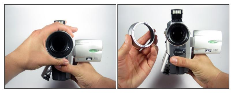
To remove the camcorder lens hood, twist the hood to counterclockwise and it will come loose, then pull towards you.
