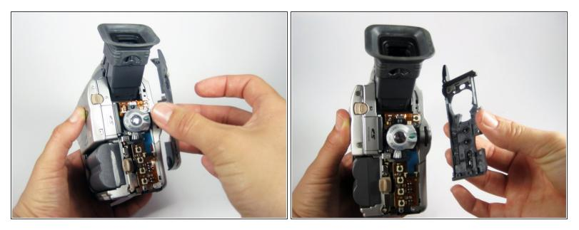
• Remove the plastic cover from the rear of the camcorder by gently pulling it towards you while holding the camera as shown.
