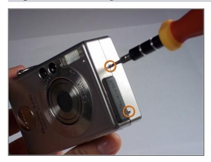
Remove two 2.4mm Phillips screws from the right side of the camera.
