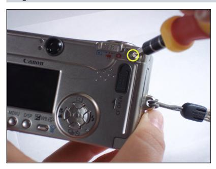
Remove one 1.6mm Phillips screw from the above the CF open button on back of the camera.
