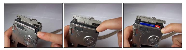
• Push down on the black square button next to the memory card slot. This will release the memory card from the slot.
