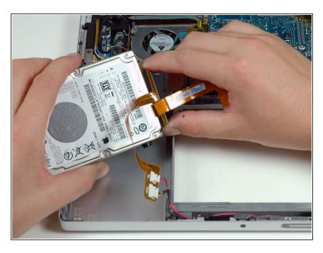
Lift up the hard drive with one hand and use your other hand to disconnect the hard drive cable.
