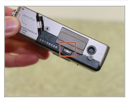
Locate the battery door marked "BATT" on the bottom of the camera.
