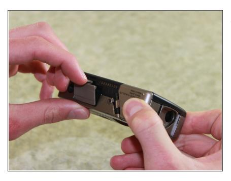
Pull the battery door tab upward and press in the direction indicated by the arrow on the tab.
