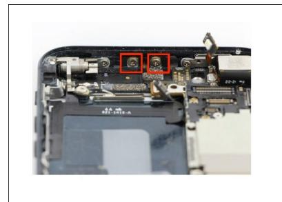
• At the top of the frame, remove the two 1.3mm Phillips screws holding the cellular service and GPS antenna's against the frame.
