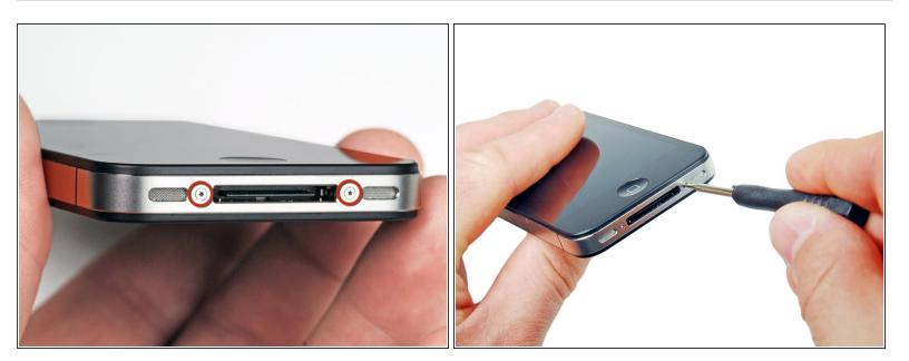
Use the Pentalobe screwdriver to remove the two 3.6 mm Pentalobe screws near the dock connector.
