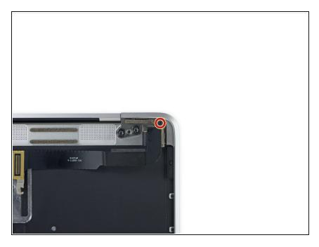
Remove the single 4.3 mm Phillips #00 screw securing the USB-C port ribbon cable.
