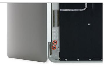
• Remove the four 4.8 mm T8 Torx screws securing the display hinges.
