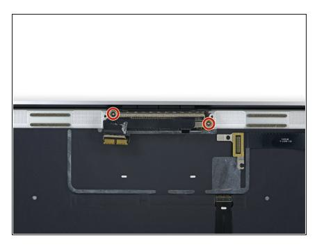
Remove the two 3.3 mm T5 Torx screws securing the display cable assembly.
