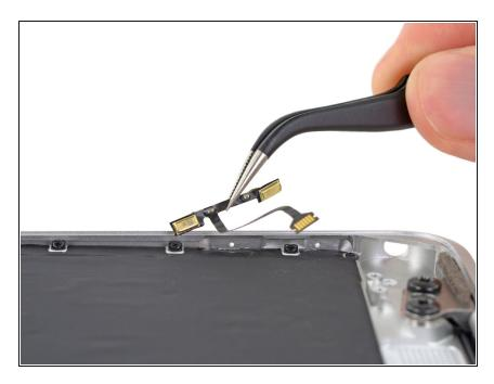
Remove the dual microphone assembly.
