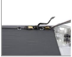
• Use a fine-tip probe or pick to gently peel the dual microphone assembly away from the case.
