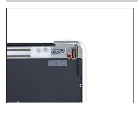
Remove the single 2.9 mm T3 Torx screw securing the USB-C port to the upper case.
