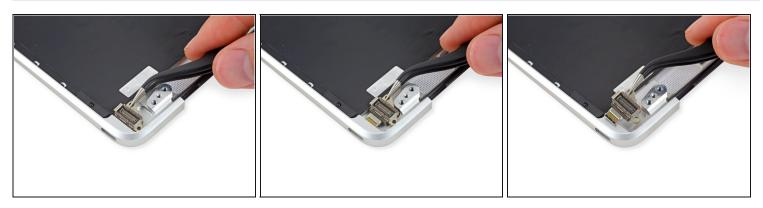
• Slide the USB-C port out of its recess in the upper case, and remove the USB-C port.
