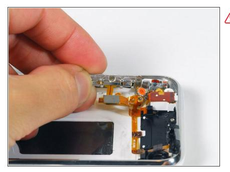
Lift the volume button circuitry away from the side of the iPhone, and carefully peel up the orange ribbon cable from the rear case. The cable is thin and easily damaged.
