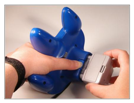
Remove the Rumble Pak from the controller by pressing the release button and pulling the Rumble Pak out.
