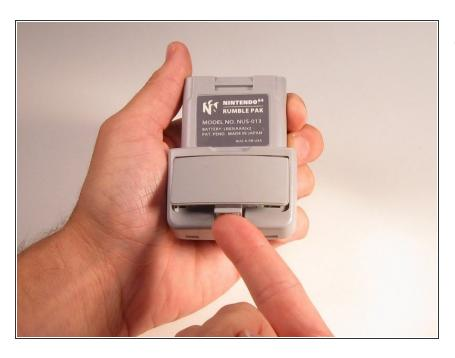
Remove the battery cover from the Rumble Pak by pressing the tab and pulling the cover up.
