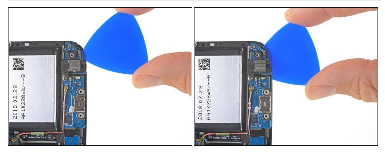
Insert an opening pick about 0.5 inches (~12mm) under the bottom corner of the display, near the headphone jack.
