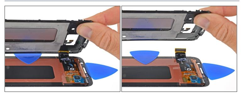
Route the display's flex cable through its hole in the frame in order to fully separate the right edge of the display.
