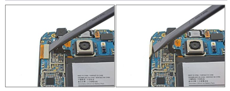
• Use the flat end of a spudger to disconnect the display assembly cable from the motherboard.
