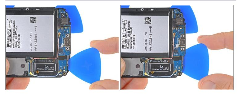
Insert an opening pick about 0.5 inches (~12mm) under the opposite bottom corner of the display.
