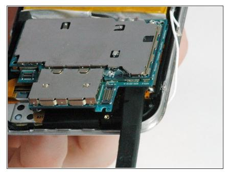
In a similar manner, slide a spudger beneath the logic board where the camera was. Again, don't lift up too far yet as there are still four attached connectors on the bottom of the logic board.
