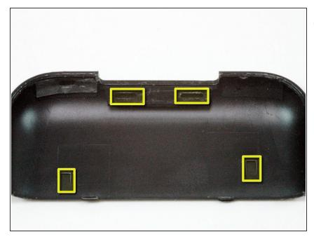
This image shows the two tabs and two catches located on the underside of the antenna cover. The two tabs at the top of the image must be pushed towards the black cover to release them.
