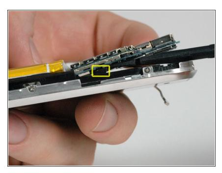
Go to the other side of the logic board and use a spudger to disconnect the touch sensor cable on the under side of the logic board.
