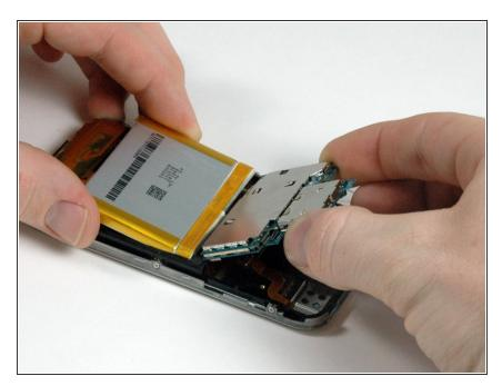
Hold both the battery and the logic board assembly and slide both parts away from the orange antenna and out of the iPhone.
