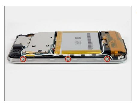
Rotate the iPhone 90 degrees and remove the three Phillips #00 screws from the side of the iPhone.
