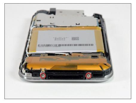
Rotate the iPhone 90 degrees and remove the two Phillips #00 screws from the bottom of the iPhone.
