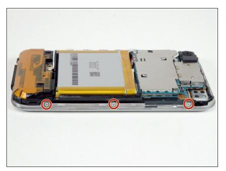
Remove the three Phillips #00 screws securing the front bezel to the iPhone.
