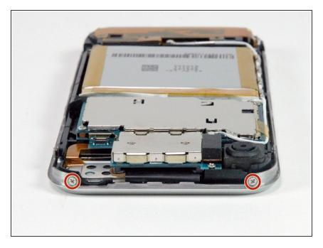
Rotate the iPhone 90 degrees and remove the two Phillips #00 screws from the top of the iPhone.
