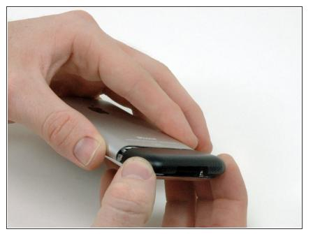
Grasp the antenna cover on either side and slide it up and away from the iPhone. This requires some force. If it does not come free, ensure that the antenna cover is lifted up enough to free the catches.
