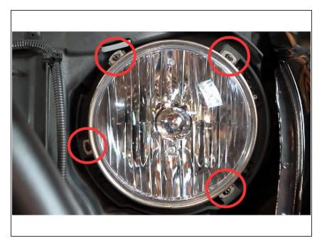
Remove the four (4) screws that are holding the metal bracket ring around the headlights.
