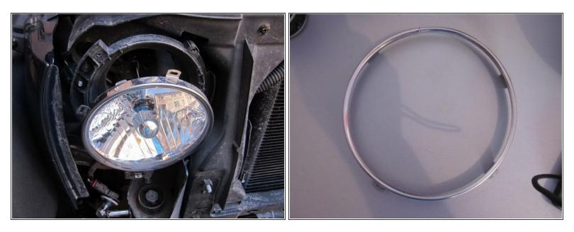
Remove the metal bracket ring.
