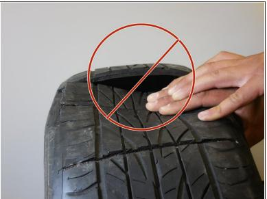
Cut across the tire using a knife creating a groove approximately the width of the tread.
