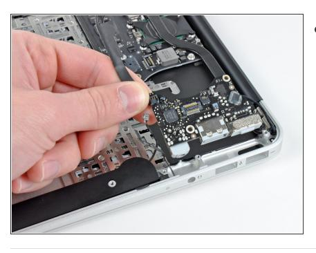
Carefully lift the I/O board from its edge nearest the logic board and remove it from the upper case.
