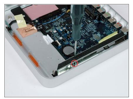
Put the screwdriver through the hole in the metal shield next to the battery, and remove the T8 torx screw concealed within.
