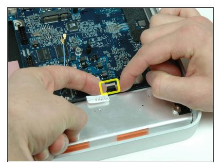
Disconnect the IR cable from the logic board.
