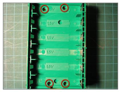
Remove the four screws in the battery compartment. These hold the yellow top on.
