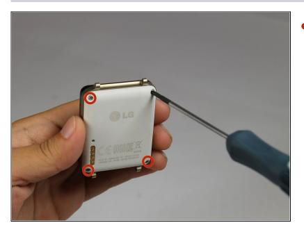
Use the T5 Torx screwdriver to unscrew the four silver 2mm x 3mm T5 screws that hold the back cover in place.
