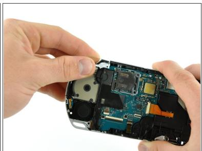
Remove both trigger buttons by lifting them off the PSP 300xc.
