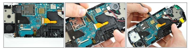
Use your fingernail or the edge of a spudger to flip up the retaining flap on the UMD drive ribbon socket.
