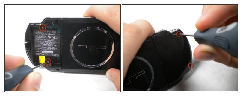
• Remove four Phillips screws from the back of the PSP.
