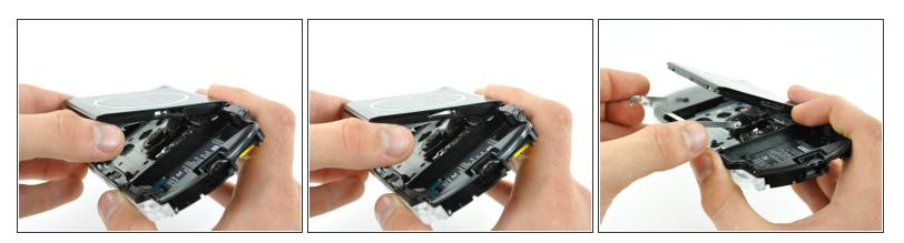
Slide the UMD brace toward the top of the UMD door until the brace disconnects from the door. Remove the brace.
