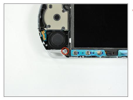
Remove a single Phillips screw securing the home bar to the PSP 300xc.
