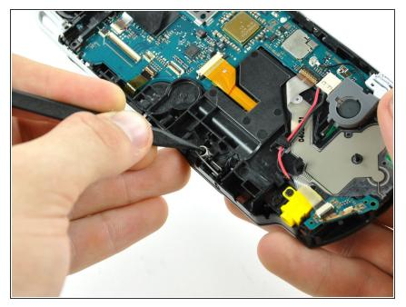
• Using the pointed end of a spudger, pull the UMD door spring to the left, and remove it from the PSP.
