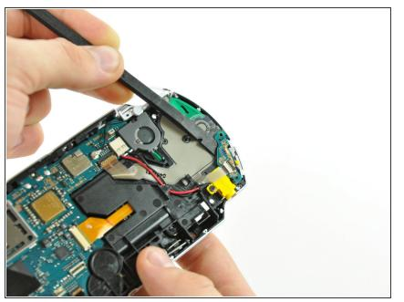
Using the flat edge of a spudger, pry the power board away from the PSP 300xc.
