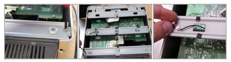
Once you have the cover off, you will need to remove the 3 metal bars that are placed across the device. Be careful with the middle section, there is a wire attached to the screw that you will need to slide through the slot in the metal bar.
