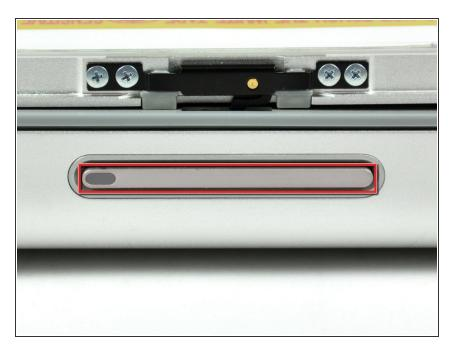
Press the display latch release and open the display slightly.
