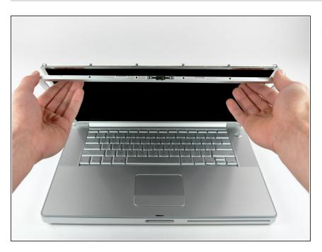
Push the LCD away from the front display bezel near its top edge.
