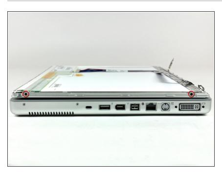
Remove the two small black Phillips screws from both sides of the display (four screws total).
