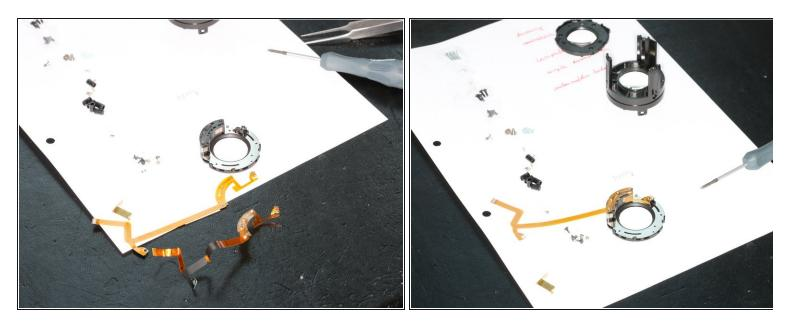
• Resolder new cable for the aperture plate
