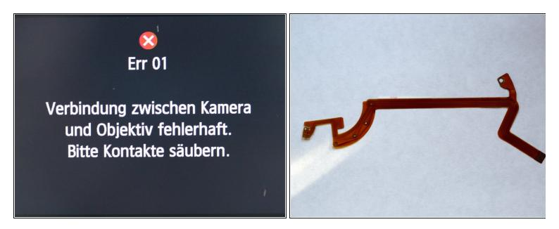
• Here is the problem with this camera and the needed replacement part is shown.
