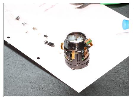
Dismantle aperture plate and IS assembly
