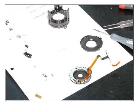
• Unsolder old flex cable for the aperture plate
