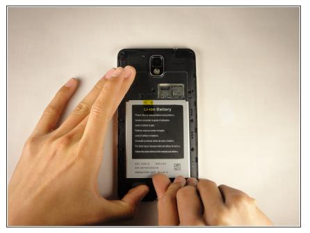
• Using either your thumb or an iFixit opening tool, remove the battery and set it aside.
