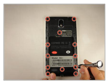
Unscrew the twelve 3 mm screws from the back panel using a Phillips #00 screwdriver.
