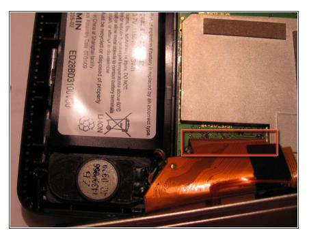
Disconnect ribbon cable from logic board.
