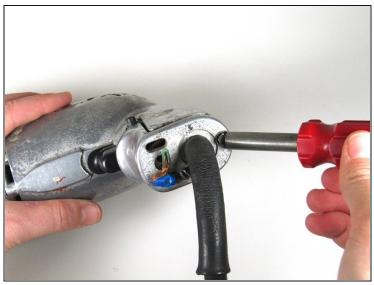
• Use the socket wrench to remove the 0.5" length screw from the bottom of the handle.
