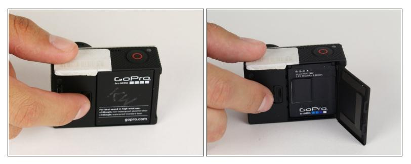
• Pull back on the tab on the back of GoPro to open the battery cover.
