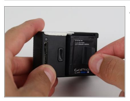
• Pull the battery out using the tab.
