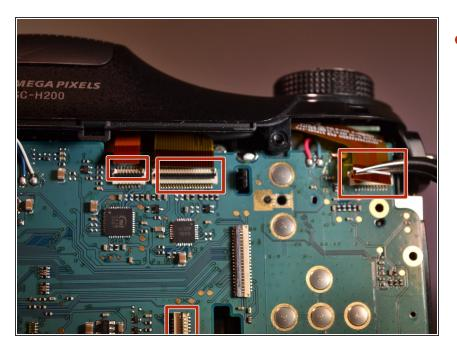
Disconnect the four amber-colored ribbon cables from the motherboard using tweezers.
