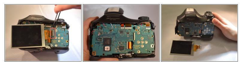
• Using tweezers, remove the LCD with the ribbon cable and set aside.
