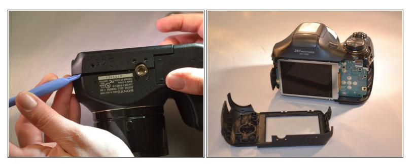
• Remove the back panel (the LCD and motherboard are exposed).
