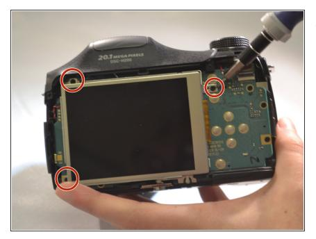
Using a screwdriver, remove the three 4mm screws that attach the LCD to the camera motherboard. (The LCD is contained in a holding plate, attached to the motherboard with a ribbon cable.)
