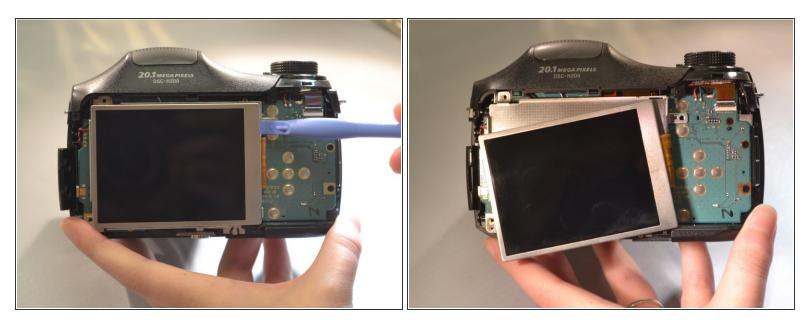
• Lift the holding plate away from the motherboard and set aside.
