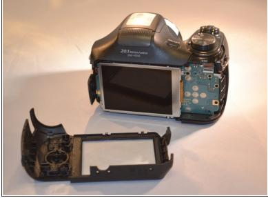
Remove the back panel (the LCD and motherboard are exposed).
