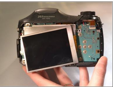
Lift the holding plate away from the motherboard and set aside.
