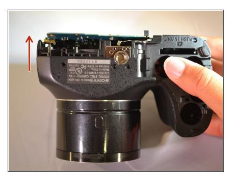
Lift the motherboard away from the camera body (the tripod port is exposed)
