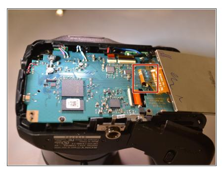
Using tweezers, open the LCD ribbon port by lifting the black hinge.
