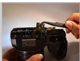
• Using tweezers, lift the tripod port up and away from the camera body
