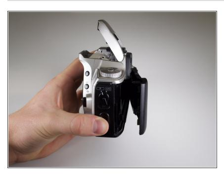
Open the back-cover of the camera using the back-cover release found on the lower right side of the camera.
