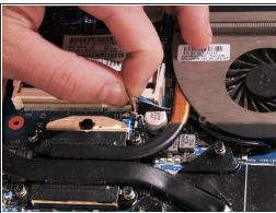
Unplug the second fan assembly cable by carefully pulling it upwards.
