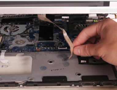
Gently pull the white connector shown in the picture towards you to disconnect it from the system board.
