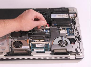
• Disconnect the multi-colored battery cable from the main assembly by gently pulling upward on it.
