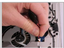
• Unplug CMOS battery by gently pulling upwards on it's cable.
