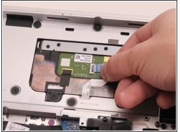
Remove the first connector by lifting the white clamp with a Flathead screwdriver and pulling the connector to your right.
