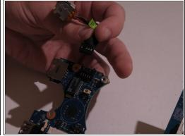
Detach the power connector by pulling it away from the motherboard.
