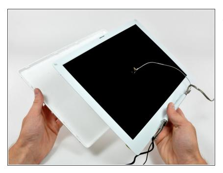
Lift the rear bezel off the display.
