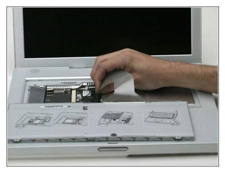
Pull the keyboard cable up from the logic board, holding the cable as close to the connector as possible.
